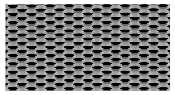
LW Pitch:19.05mmStrand Width:3.00mmSW Pitch:7.62mmThickness:0.70mmWeight:4.55 kg / m2Open Area:21%
